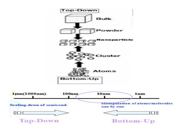
Figure 2: Schematic representation of 'top-down' and 'bottom-up' approaches for synthesis of nanoscale materials.
